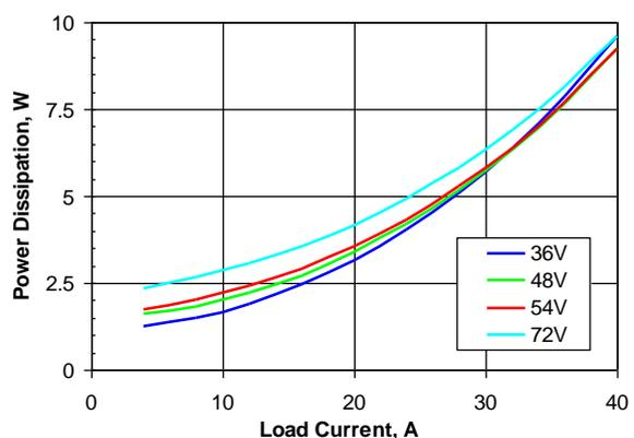
Figure 5. Power dissipation vs. load current and ambient temperature for SQE48T40015 converter mounted vertically with  $V_{in} = 48\text{ V}$  and air flowing from pin 3 to pin 1 at a rate of 200 LFM (1.0 m/s).
