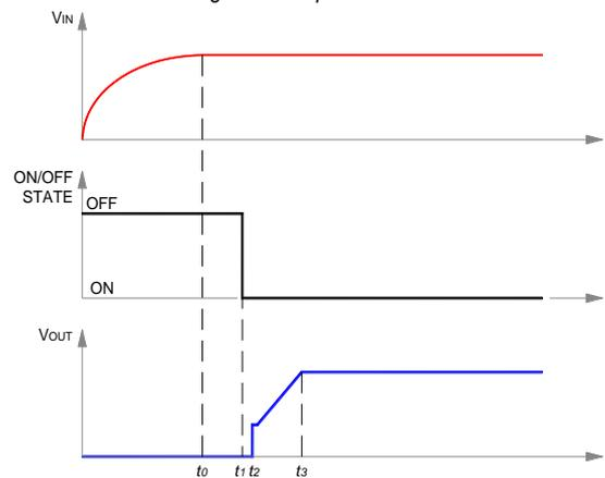
**Scenario #3: Turn-off and Restart Using ON/OFF Pin**
