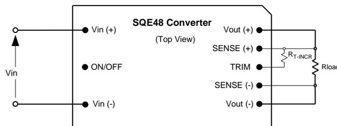
To decrease the output voltage (Fig. D), a trim resistor, R<sub>T-DECR</sub>, should be connected between the TRIM (Pin 6) and SENSE(-) (Pin 5), with a value of:
