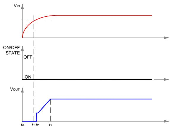
**Scenario #2: Initial Startup Using ON/OFF Pin**
