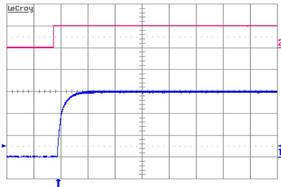
Figure 8. Output voltage response to load current step-change (20 A – 30 A – 20 A) at  $V_{in} = 48\text{ V}$ . Top trace: output voltage (100 mV/div.). Bottom trace: load current (10 A/div.). Current slew rate: 0.1 A/ $\mu\text{s}$ .  $C_o = 1\text{ }\mu\text{F}$  ceramic. Time scale: 0.2ms/div.
