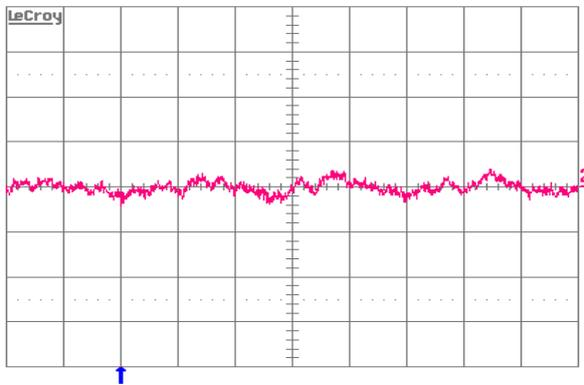
Figure 13. Input reflected-ripple-current,  $i_c$  (100 mA/div.), measured at input terminals at full rated load current and  $V_{in} = 48$  V. Refer to Figure 11 for test setup. Time scale: 1  $\mu$ s/div.
