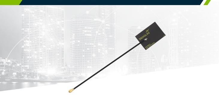
The AccuraUWB FXUWB10 flexible polymer antenna, at 35\*24.5\*0.2 mm, is a small form factor, ultra-thin Ultra-Wideband (UWB) antenna with high efficiencies across the pulsed UWB communications operational bands. It is assembled by a simple "peel and stick" process, attaching securely to non-metal surfaces via 3M adhesive. It enables designers to use only one antenna that covers all available UWB commercial bands, namely bands 1 through 15 simultaneously.
