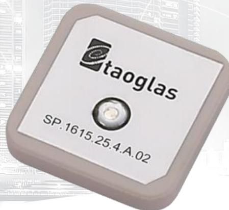
This miniaturized 25mm square ceramic patch antenna is mounted via pin and double-sided adhesive and is the optimal embedded antenna solution for mobile Globalstar applications.
