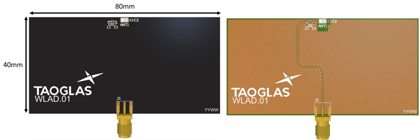
Top Side (WLA.01 placement on 80x40mm PCB)
