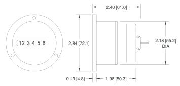
Mounting holes: For #4 screws on 2.44" [62.0] B.C. and #6 screws on 2.53" [64.3] B.C. Panel cutout: 2.21" [56.1] Dia.
