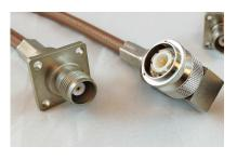
Standard TNC Plug connectors can mate to a Keyed TNC Jack connector, but standard TNC Jack connectors will not mate to a Keyed TNC Plug.
