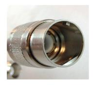
Keyed TNC Plug connectors have an extended length coupling nut that features a flat and a keying rib that can be located at up to 24 different angles, or keyed positions, from the flat feature.
